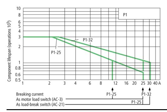
For utilisation category AC-4 (extreme load: 100 % inching, reversing or plugging) The blocked rotor current of the motor should not exceed the rated current of the switch for AC-21A to ensure a reasonable device lifespan.
